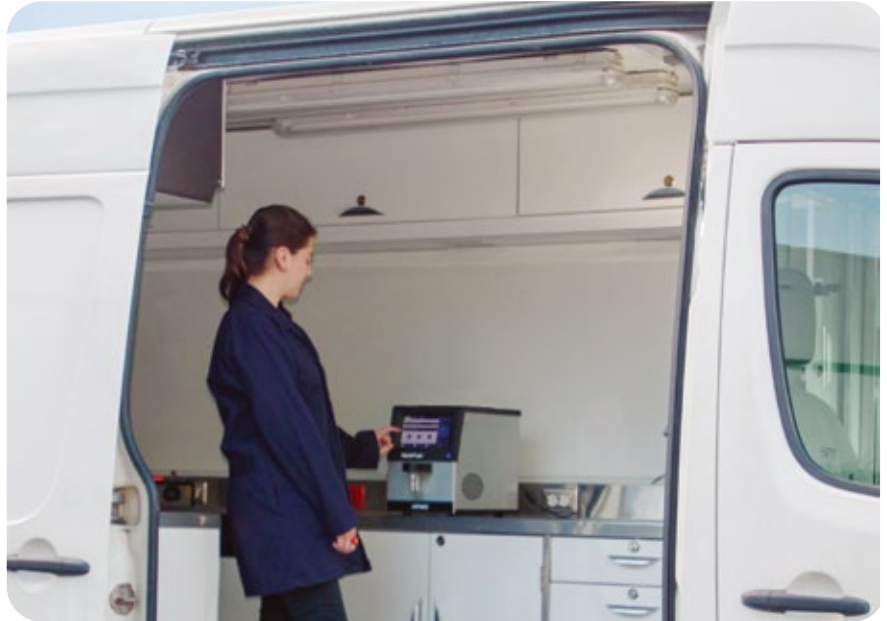
Mobile Lab is enclosed climate controlled lab with ambient temperature and humidity within product specification to obtain desired performance.
